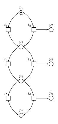
Figure 4: A net system with a large marking complete prefix.
