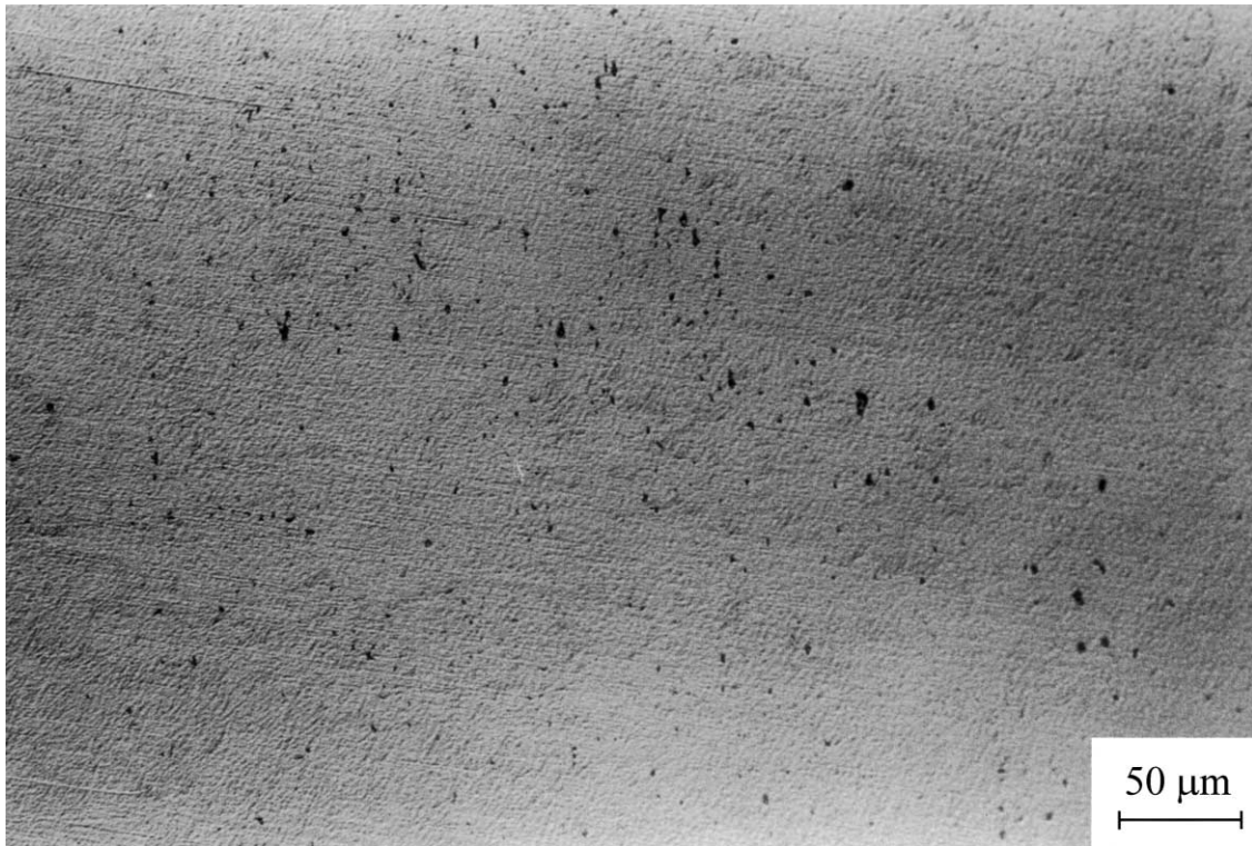
Fig. 4. Optical micrograph from wear zone of polyethylene disk, test 1.
