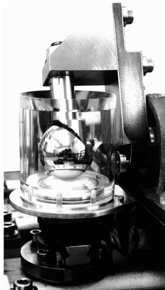
Fig. 1. Close-up of three-axis knee wear simulator with ball-on-flat contact.
