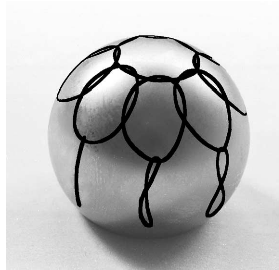
Fig. 9. Grooves engraved onto 28 mm dia. CoCr head in BRM simulator having zero-offset rotation-prevention lever. Points selected and viewing angle set as in Fig. 8 (a).
