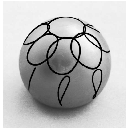
Fig. 10. Grooves engraved onto 28 mm dia. CoCr head in BRM simulator having rotation-prevention lever with 20 mm offset and rotation-prevention post with 65 mm distance from the centre of head. Engraving cup was same as in Fig. 9.
