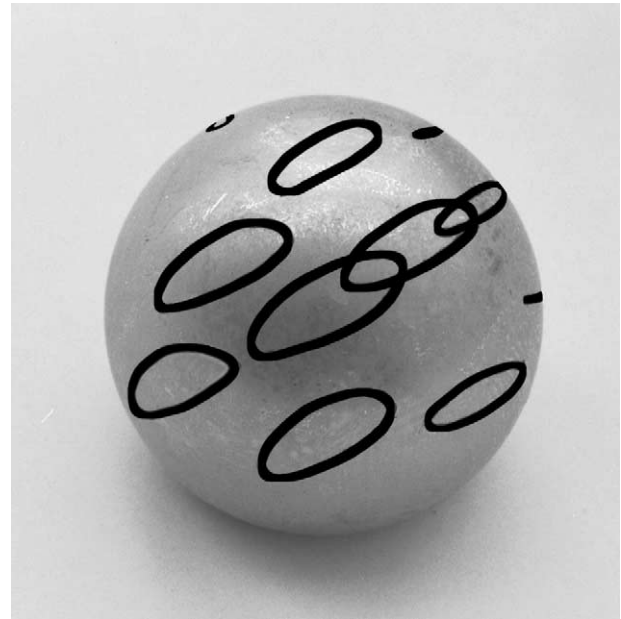
Fig. 7. Grooves engraved onto 28mm dia. CoCr head in HUT-3 simulator. Points selected and viewing angle set as in Fig. 6(a). Grooves accentuated with ink, reflections repressed.
