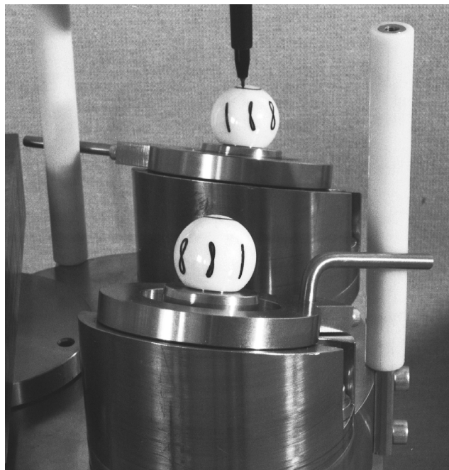
Fig. 5. Additional verification of head tracks in BRM simulator using 28 mm dia. zirconia heads and stationary drawing pen. Station in front has zero-offset lever; straight line is parallel to neck axis, and symmetric figure of eight is on equator. Station in background has offset lever; straight line is inclined relative to neck axis, and symmetric figure of eight is elevated relative to equator. Note also latitudinal ( 67^\circ ) force tracks.
