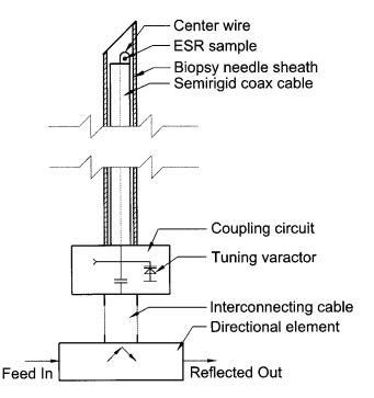
**Figure 2.** Microwave parts of an ESR probe, adapted for use with biopsy needles.
