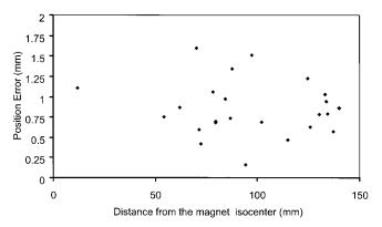
**Figure 3.** Position error as a function of the distance from the magnet isocenter.
