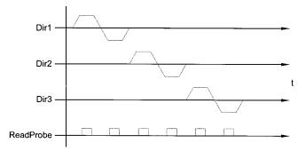
Figure 1. Position encoding gradient sequence for ESR magnetometer.
