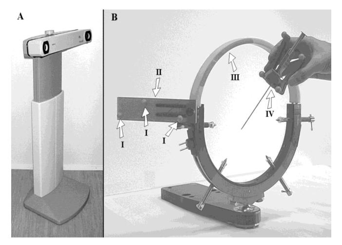
Figure 2. Navigator elements. A: Camera head on navigator stand. B: Frame with patient tracker (I, II) and detachable upper part (III). Also shown is the instrument tracker (IV).
