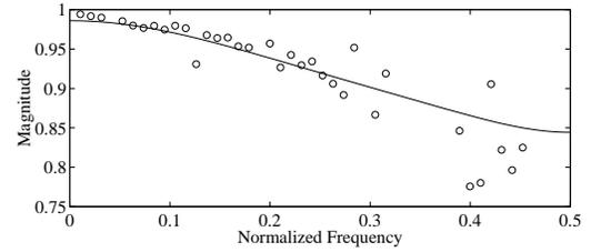
Figure 4: The biquad filter magnitude response (solid curve) compared with the desired gains of the harmonics (circles) of a lute tone (first string, third fret,  $f_0 = 464$  Hz).
