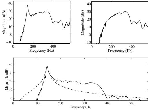
Figure 3: The extraction of a body mode from a lute excitation signal. The body mode occurs at  $f_1 = 144$  Hz (top-left), and it is effectively removed by the notch filter of Eq. (1) (top-right). The resonator of Eq. (2) reconstructs the body resonance (bottom).
