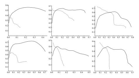
**Fig. 3.** Recall–precision plots (x-axis: recall; y-axis: precision) using the keyword feature with (solid curve) and without (dashed curve) the MPEG-7 descriptors. The *a priori* probability of the class is shown with a dotted line. Used classes were (top row, left-to-right) **faces**, **cars**, **planes**, (bottom row) **sunsets**, **horses**, and **traffic signs**.
