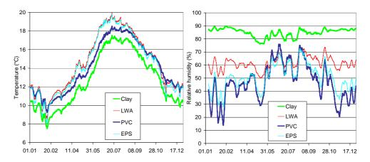
**Fig. 14.** Crawl space air temperature 24-hour moving average (left) and relative humidity weekly moving average (right) with different ground covers; the air change rate is 0.5 ach.
