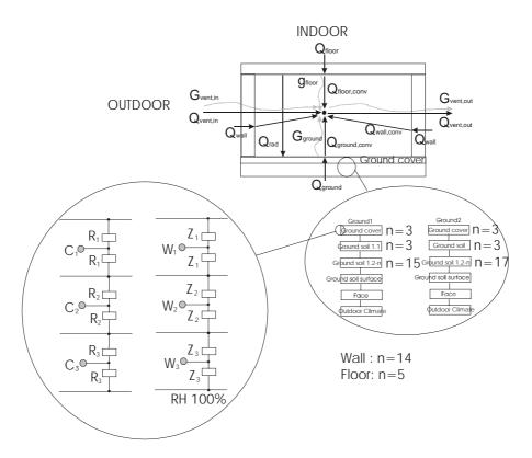
**Fig. 3.** RC-network model of the crawl space: Q – heat flow, g – moisture flow, W – moisture content by volume, Z – diffusive moisture resistance, C – volumetric heat capacity, R – thermal resistance, n – number of calculated nodes.
