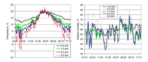
**Fig. 9.** Calculated 24-hour moving average air temperature (left) and weekly moving averages of RH (right) in the crawl space at various air change rates; the ground is covered with 17 cm LWA.
