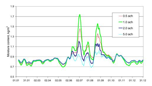
Fig. 12. Moisture content (weekly moving average) inside the LWA at a 5 cm depth.
