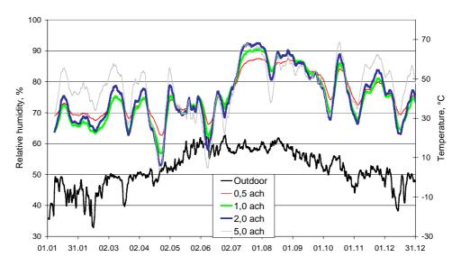
**Fig. 13.** Relative humidity and outdoor temperature in the cold crawl space when the weather data of the Finnish test-year for energy calculations (1979) is used.
