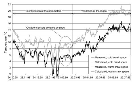
**Fig. 4.** Calculated and measured temperatures in the crawl spaces. The air change rate in both calculations is 1.1 ach (24-hour moving averages).
