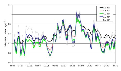
$\textbf{Fig. 10.} \ \ \text{Moisture content weekly moving average inside the LWA at the depth of 6.7\,cm for different air change rates.}$
