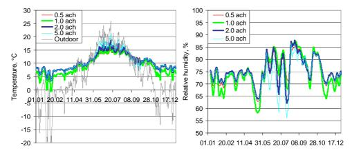
**Fig. 11.** Crawl space air temperature 24-hour moving average (left) and relative humidity weekly moving average (right) for various air change rates; the ground is covered with a 15 cm layer of LWA.
