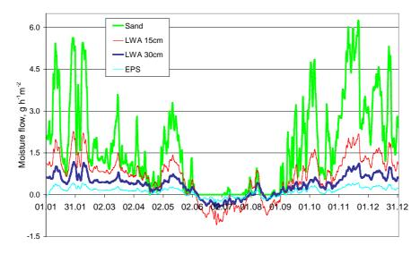
**Fig. 17.** Moisture flow from the ground (evaporation rate in the case of sand); positive values indicate evaporation and negative values moisture flow from the air to the ground (24-hour moving average).
