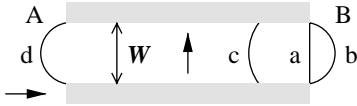
Fig. 1. Equilibrium position of the A–B interface in the channel at different pressures: (a) p = p_0 , (b) p > p_0 , (c,d) p < p_0 . The thick arrows denote orientation of \hat{l} vector when there is A phase in the respective regions.
