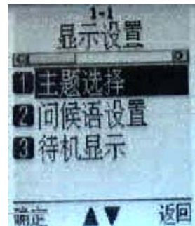
Figure 54. Amoisonic A8+ vertical menu with horizontal scrollbar
