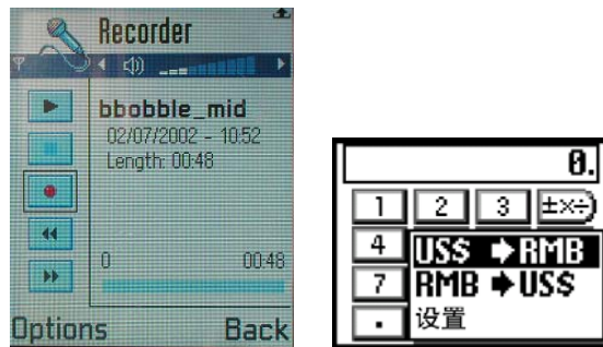
Figure 55. Screen buttons in Nokia 7650 recorder, and in Sony CMD Z28 calculator 118
