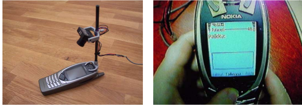
Figure 98. Mobile phone usability test observation camera 214 attachment and the camera image as seen on the observation monitor display
