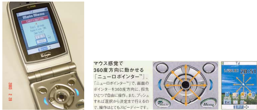
Figure 65. 360 degree 'Neuropointer' UI in NEC N2051
